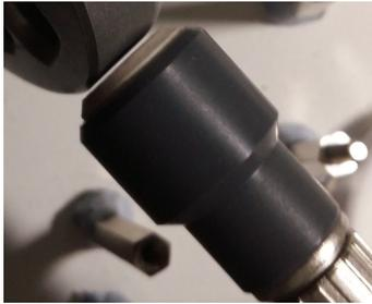
Physical contact with the specimen is not necessary, allowing to design systems capable of performing millions of measurements. This feature prevents sensor damage and abrasion. The automation has to ensure the part comes close to the sensor until the output **DOK** is high, then check if the part failed the test by monitoring the output **F**.
